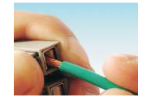
Figure2, insert the conductor into it.
