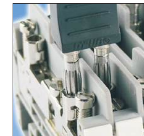
Figure 4, short-circuit plug: for short circuiting neighboring terminal blocks.
