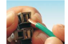
Figure1, press the upper insulation cover to open the cable entry.
