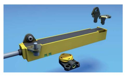
The compact Li-Q17L as well as the Li-QR14 series are built in a highly tight plastic housing, made for many aggressive ambient conditions. They are available in lengths of 50 mm to 200 mm (Li-Q17L series) resp. 25 mm (Li-QR14 series). Angled and straight mounting elements guarantee highest flexibility for mounting. The positioning element is moreover rotatable and can be oriented parallelly or crosswise to the sensor.
